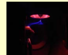
Figure 7. Corona Discharge observed in ECI/ESI LC/MS conditions
